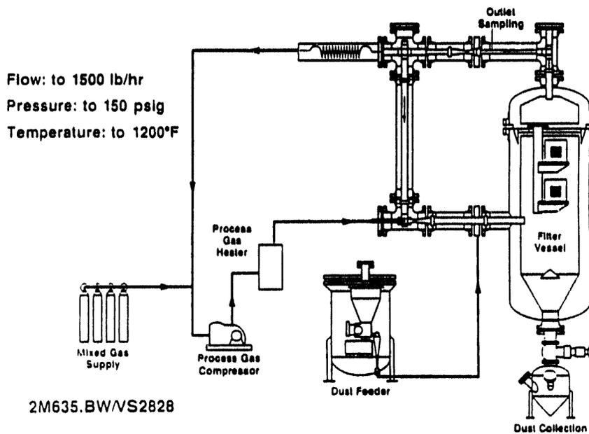
Figure 1.7b - Schematic of the Westinghouse Gasifier Simulator Test Loop
