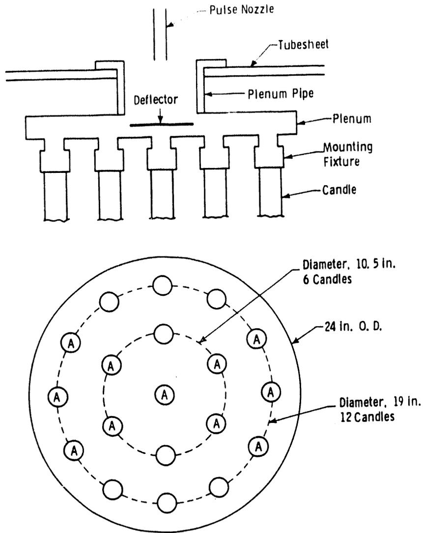
**Figure 3.3 - HTHP Candle Array Arrangement**
