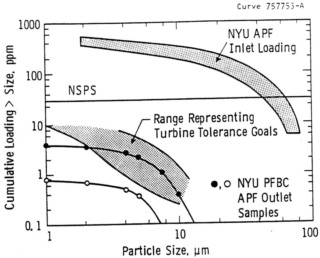
Figure 1.6 - Data Comparing Outlet Particle Size Distribution with Turbine Tolerance Goals
