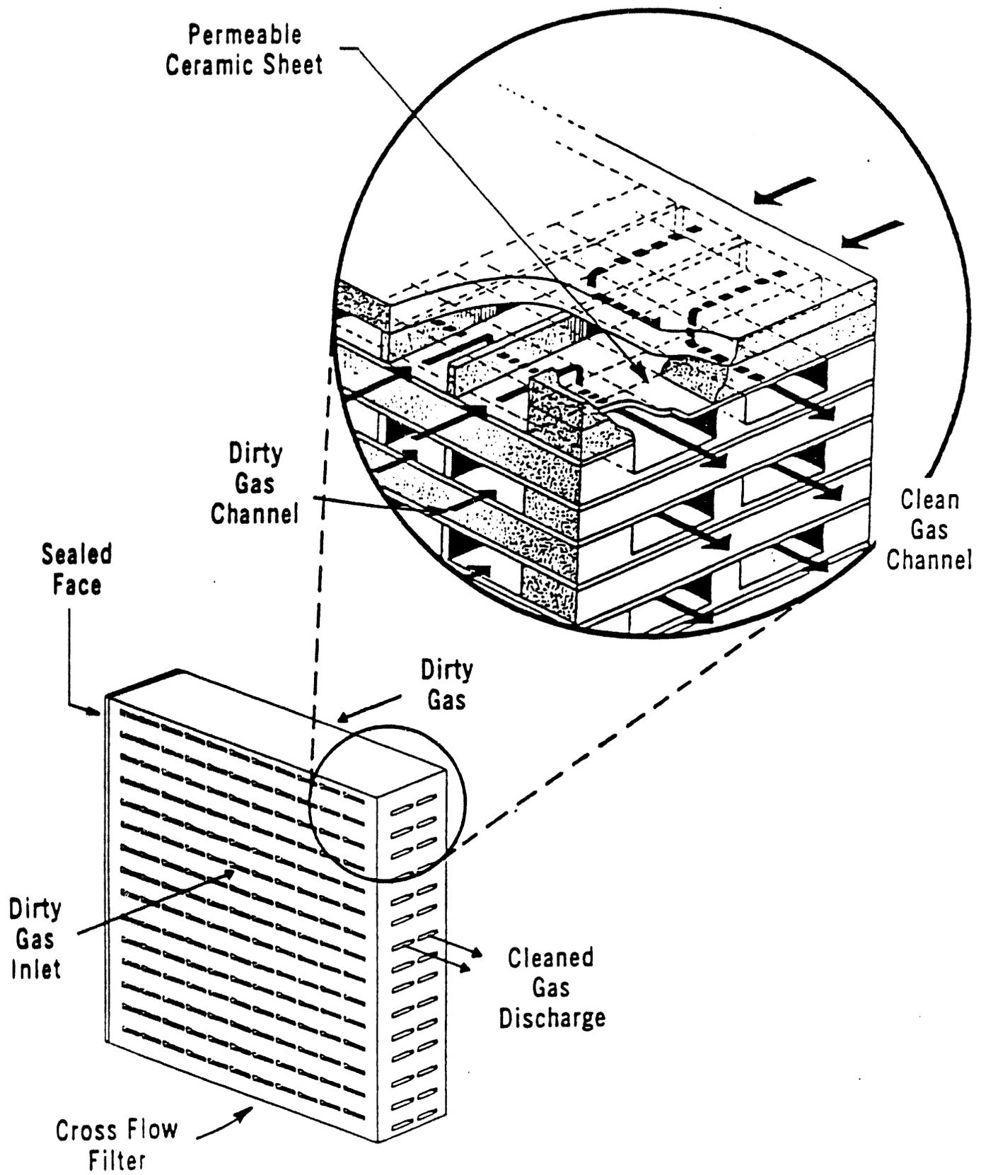
Figure 1.2 - Schematic Representation of Cross Flow Filter
