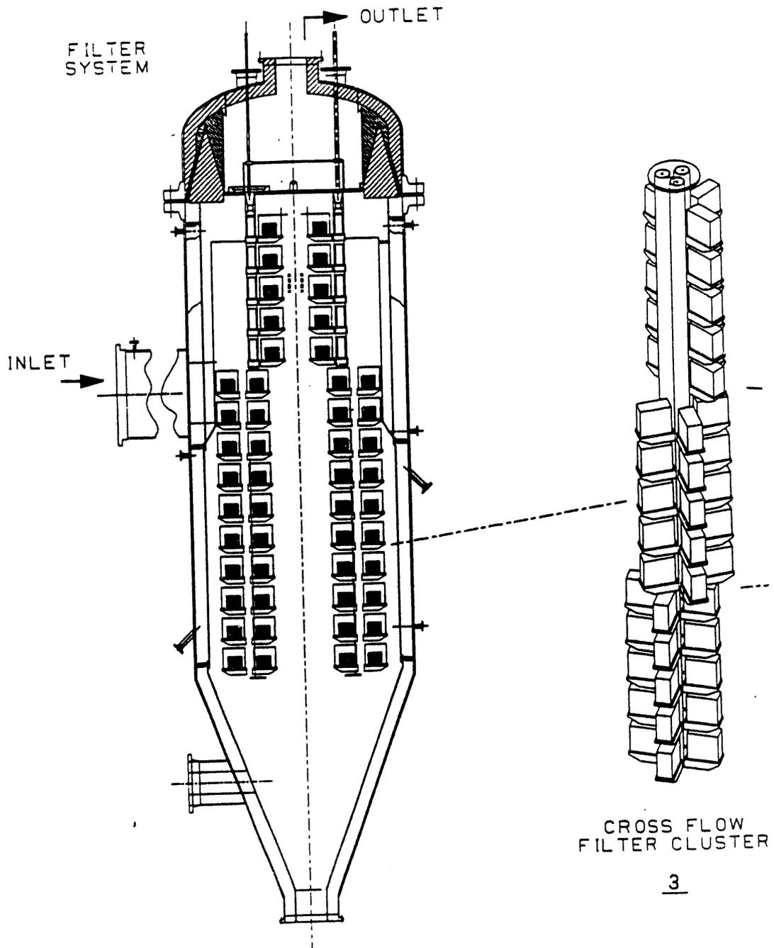
Figure 1.3 - Westinghouse Cross Flow Filter System Concept
