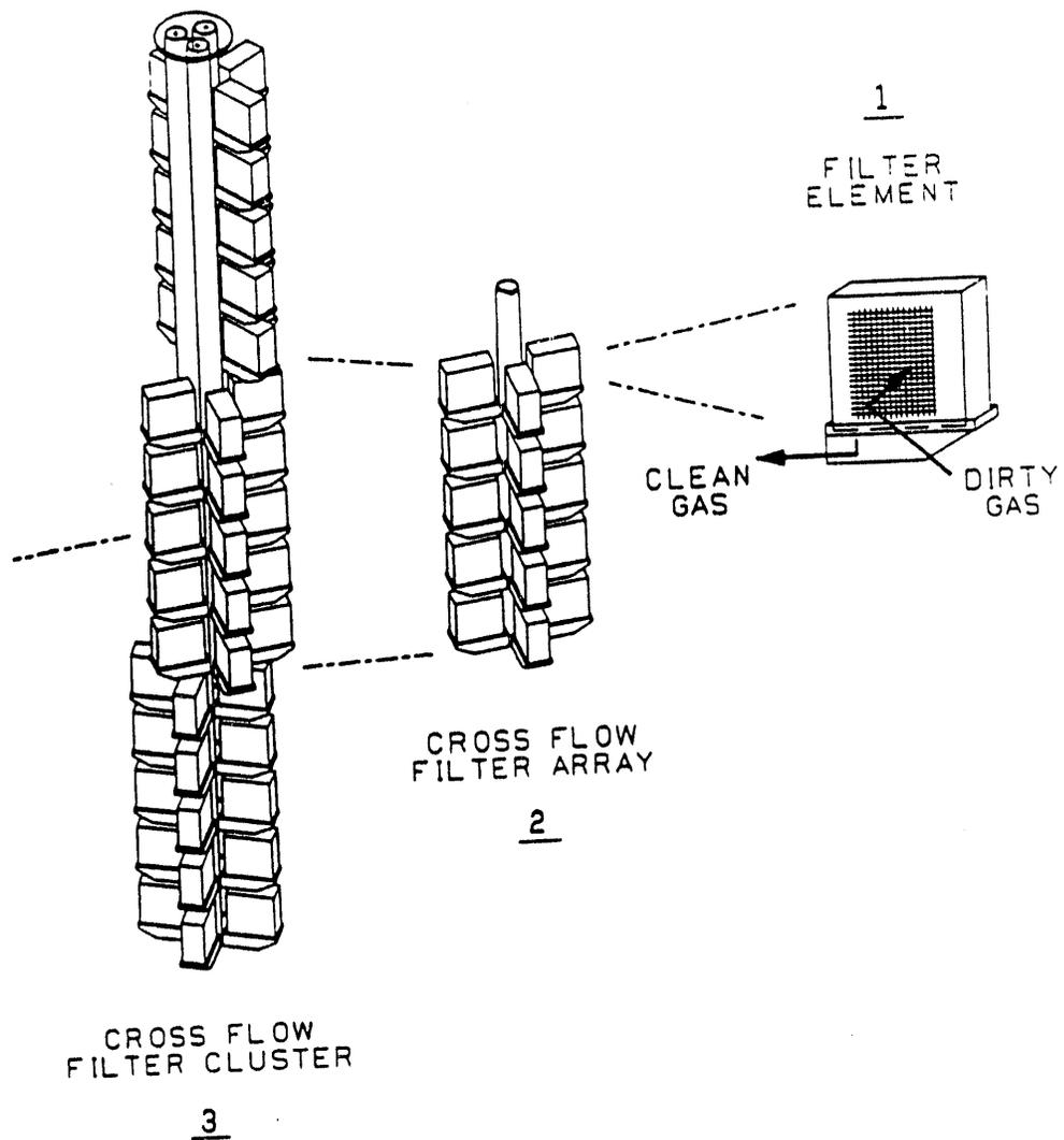
Figure 1.4 - Westinghouse Concept for Constructing Filter System from Single Cross Flow Filter Elements
