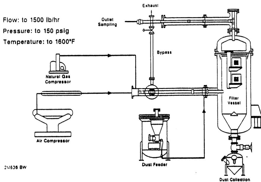
Figure 1.7a - Schematic of Westinghouse PFBC Simulator Test Loop
