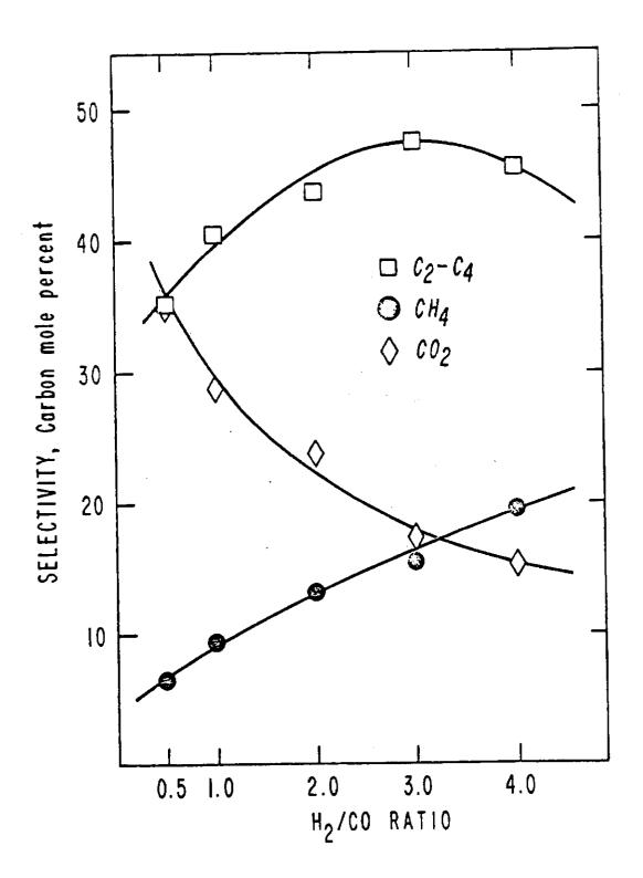
Effect of  $\rm H_2/CO$  Ratio on Product Distribution Diluted Bed, Pseudo Slurry Reactor Temperature = 503 K; Pressure = 2600 KPa; Space Velocity =  $1 \text{ cm}^3\text{g}^{-1}\text{s}^{-1}$ ; Heat Transfer Liquid Flow Rate  $(n-C16) = 0.103 \text{ cm}^3 \text{s}^{-1}$ .
