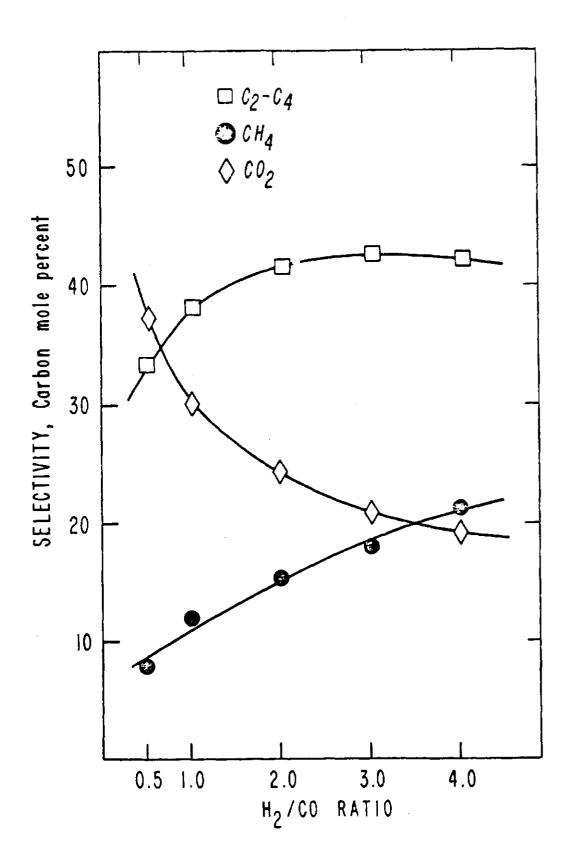
Effect of  $\rm H_2/CO$  Ratio on Product Distribution Diluted Bed, Pseudo Slurry Reactor Temperature = 503 K; Pressure = 2000 KPa; Space Velocity = 1 cm<sup>3</sup>g<sup>-1</sup>s<sup>-1</sup>; Heat Transfer Liquid Flow Rate (n-C16) = 0.103 cm<sup>3</sup>s<sup>-1</sup>.
