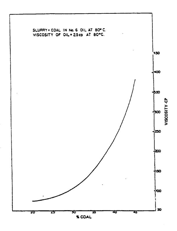
Figure 2. Viscosity of Coal/Oil Mixture; Source. (4)
