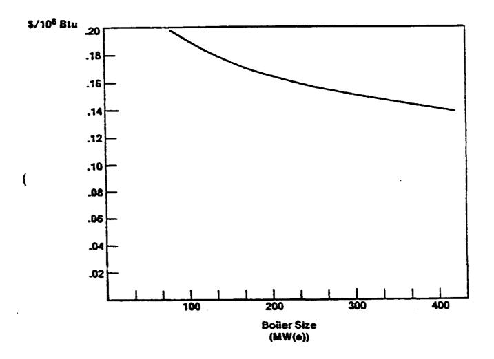
Figure 4. Boiler Conversion Costs; Source: (14).
