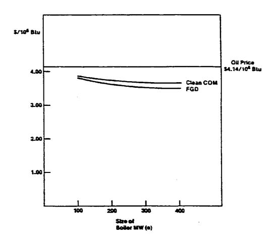
Figure 6. Cost of COM vs. Cost of Oil - Dedicated Preparation Plant; Source: (14).
