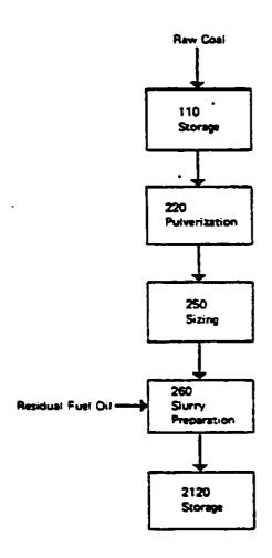
Figure 1. Flow Diagram of Coal-Oil Mixture Preparation.
