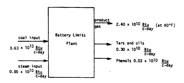
Overall plant thermal efficiency = 61%
