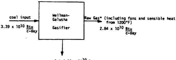
Ash 0.11 x  $10^{10} \frac{\text{Btu}}{\text{c-day}}$ Overall gasifier efficiency = 87%
