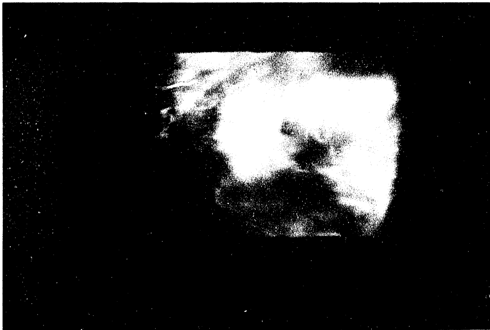
Figure 12. Indian Head flame at full load and swirl setting of 0.5.
