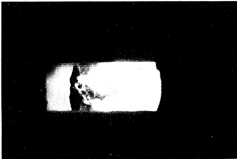
Figure 14. Indian Head flame at one-half load and swirl setting of 1.5.
