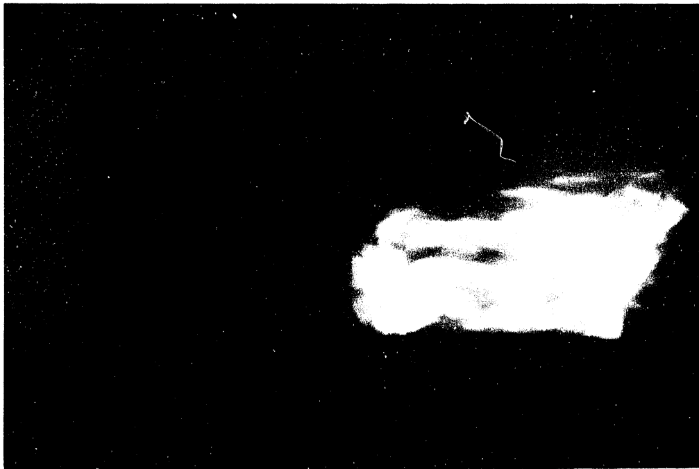
Figure 15. Indian Head flame at one-half load and swirl setting of 1.0.
