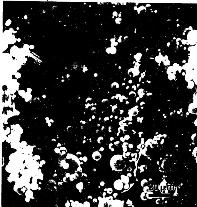
Figure 101. Scanning electron micrograph of syncoal fly ash generated at 1500°C (500x).
