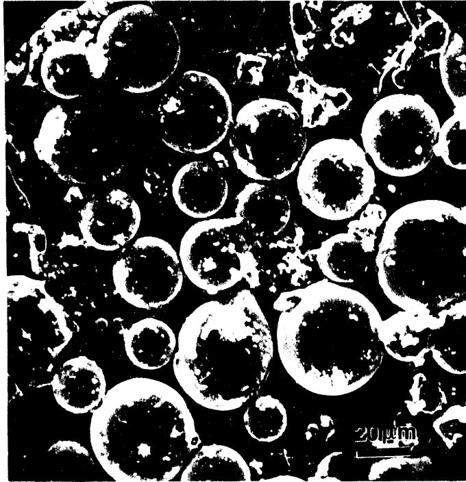
Figure 98. Scanning electron micrograph of syncoal fly ash generated at 900°C (500x).
