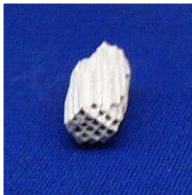
Figure 1. ZnO-coated cordierite monolith. ZnO weight loading is 40 wt%
