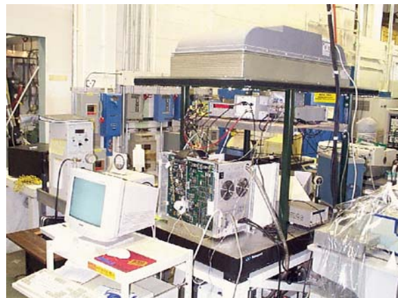
Figure 4. Real-time single particle analyzer mass spectrometer in ORNL engine lab
