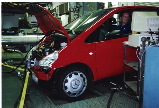
ORNL Researchers Conducting Chassis Dynamometer Tests on the Mercedes A170
