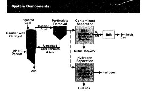
▲ Systems for the production of hydrogen or synthesis gas consist of a gasifier which converts coal or coal-derived material into a mixture of gases. A catalyst is used to increase the hydrogen concentration in the gases. After removal of particles of incompletely reacted coal or ash, the gas is separated in high-temperature membrane reactors to provide pure hydrogen or a synthesis gas free of contaminants.
