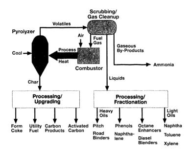
▲ Mild gasification is a less costly, coal-based alternative to traditional petroleum-based means of producing liquid and solid fuels and other non-fuel products. The coal is first fed into a pyrolyzer reactor where liquids, solids, and various volatiles are produced.
