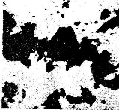
1000 X Original Coal 91 percent through 200 mesh
